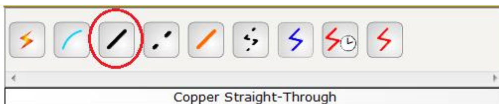
Gambar 9. Copper Straight-Through di Device-Specific Selection Box
