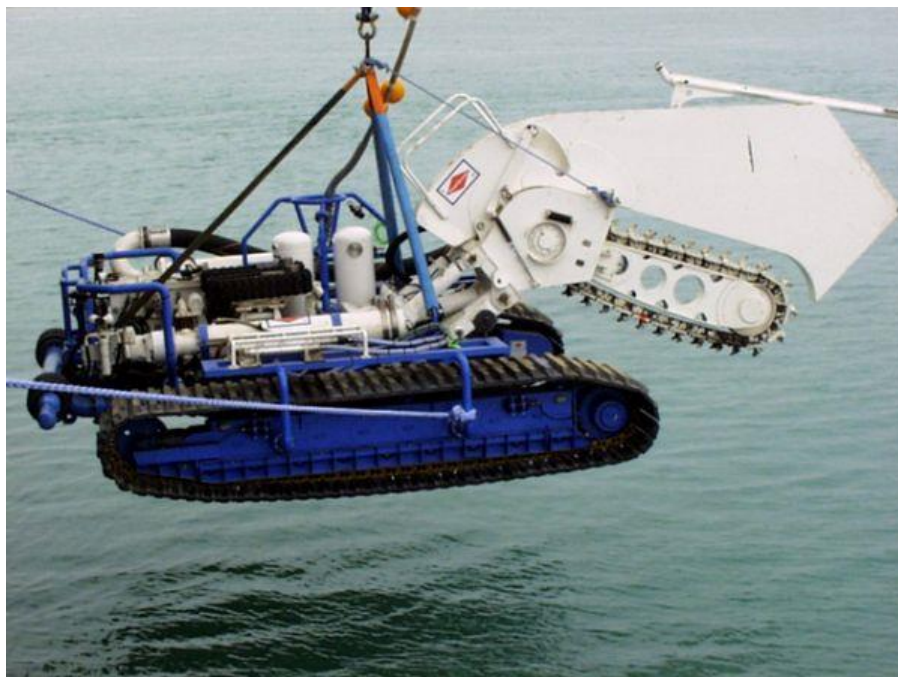
Gambar 2.7 Contoh Hydro Jet Cable Burial Machine
